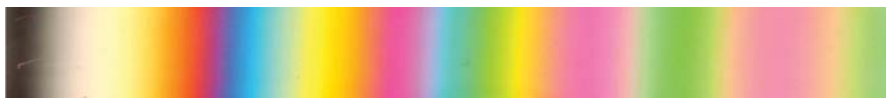
Fig. 3: Polarization colors are the same as those formed on an oil slick.
